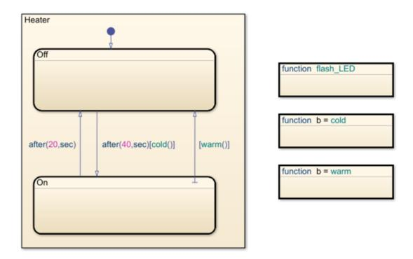
The labels on the transitions between the On and Off substates define the behavior of the bang-bang controller.
