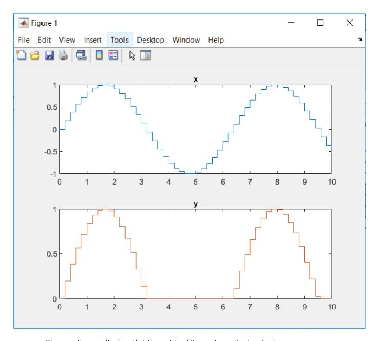
The execution results show that the rectifier filters out negative input values.
