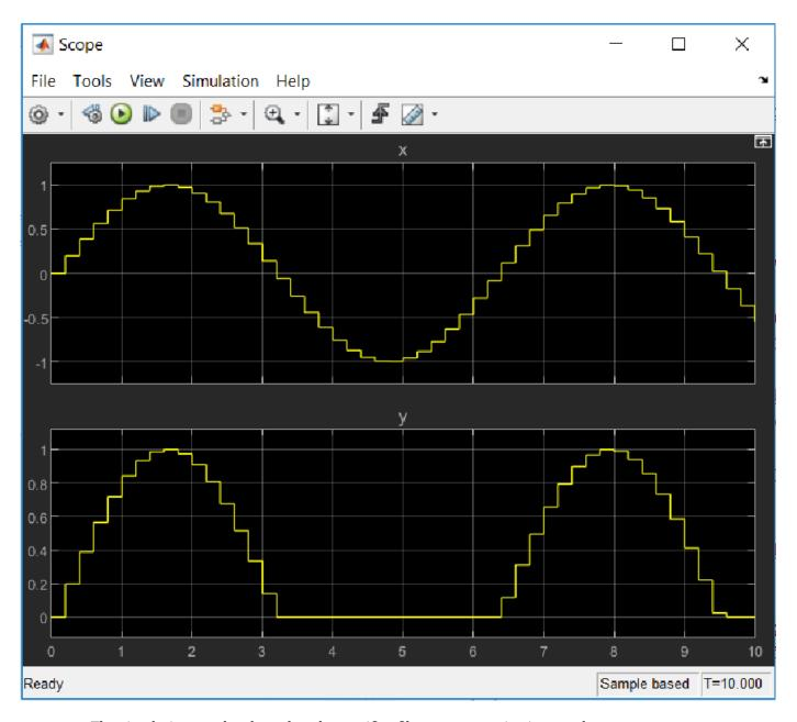
The simulation results show that the rectifier filters out negative input values.
