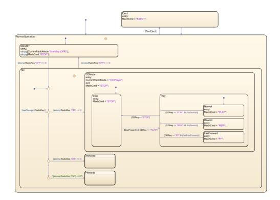
The history junctions  $\Theta$  inside the NormalOperation and ON states record the operating mode (Standby or ON) and the active subcomponent of the media player (CD player, AM radio, or FM radio) before you eject a disc or turn off the system.
