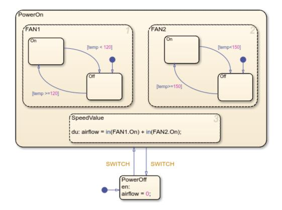
The controller operates two fans. The first fan turns on when the air temperature rises above 120 degrees. The second fan provides additional cooling when the air temperature rises above 150 degrees. The chart models these fans as parallel states FAN1 and FAN2, both of which are active when the controller is turned on. Except for their operating thresholds, the fans have an identical configuration of states and transitions that reflects the two modes of fan operation (On and Off).
