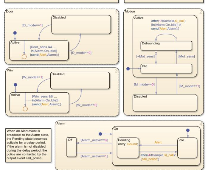
The security system consists of an alarm and three anti-intrusion sensors (a window sensor, a door sensor, and a motion detector). After the system detects an intrusion, you have a small amount of time to disable the alarm. Otherwise, the system calls the police.
