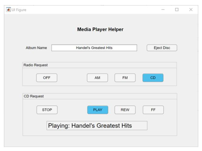
The stereo is initially in standby mode (OFF). When you select one of the Radio Request buttons, the stereo turns on the corresponding subcomponent. If you select the CD player, you can click one of the CD Request buttons to choose Play, Rewind, Fast-Forward, or Stop. You can insert or eject a disc at any point during the simulation.
